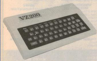
Dick Smith Electronics has introduced a new low-cost personal computer, the VZ-200. Features of the unit include a Z80A processor, eight colour graphics, sound effects, Microsoft Basic in 16K of ROM and both RF and composite video outputs for connection to a standard television set or a colour monitor.
